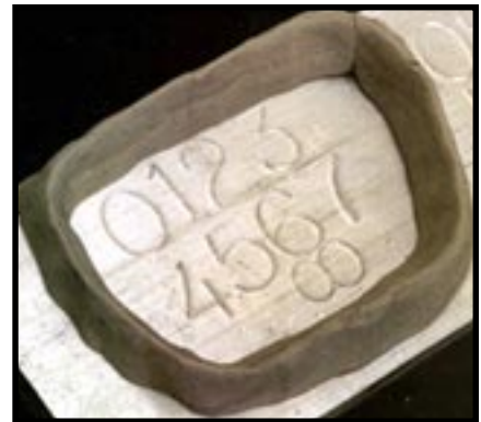
Preparation for casting stamped numbers.
