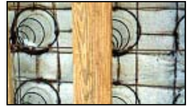
Thermally damaged box springs.
