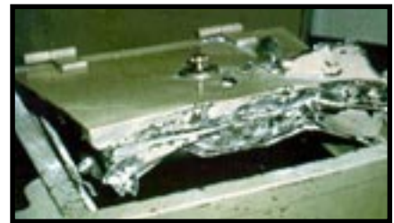
Safe insulation exposed by peeling a safe door.
